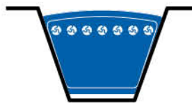
Belt wear rough grooves, slip, overload
